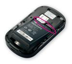
Slide the SIM card into or out of the SIM card slot, as shown. Align the metal contacts on the battery with the metal contacts in the battery compartment and press the battery into place. Replace the back cover.
